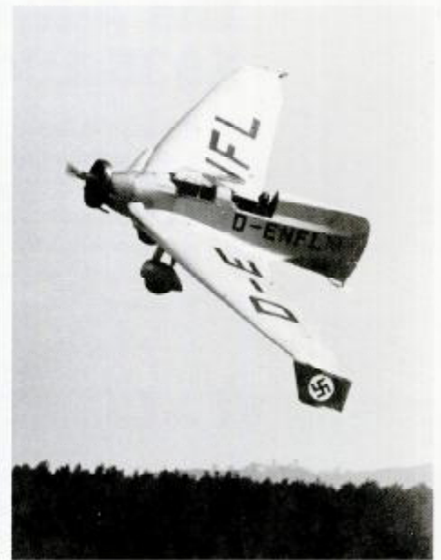
ABOVE: The Lippisch Delta IVc was tested by Heini Dittmar at Darmstadt-Griesheim between January 1937 and April 1939. It was powered by a 75 hp Pobjoy engine and had a fixed undercarriage. Also known as the DFS 39, it was transferred to the Messerschmitt plant at Augsburg where it continued flying until August 1941.
