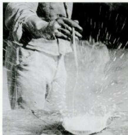
BELOW: Taken from a training film for Me 163 ground crew, this dramatic photograph shows the effect of adding a small drop of one rocket fuel component to a saucer of the other.
