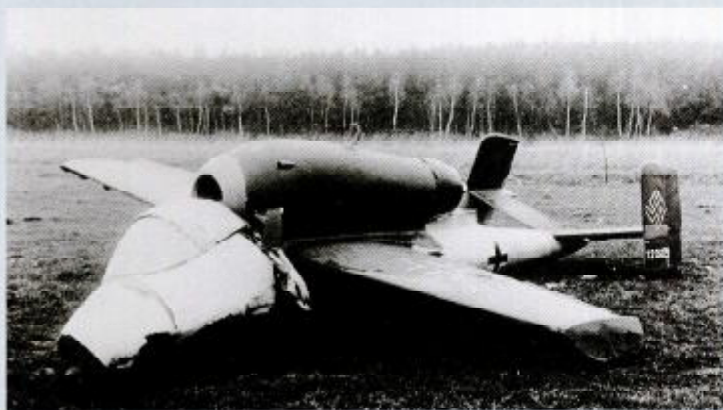
ABOVE: Because of the somewhat tricky handling characteristics of the He 162, this sight was not uncommon. This aircraft (W.Nr. 120029) made a wheels-up landing following a training flight and broke its back.
