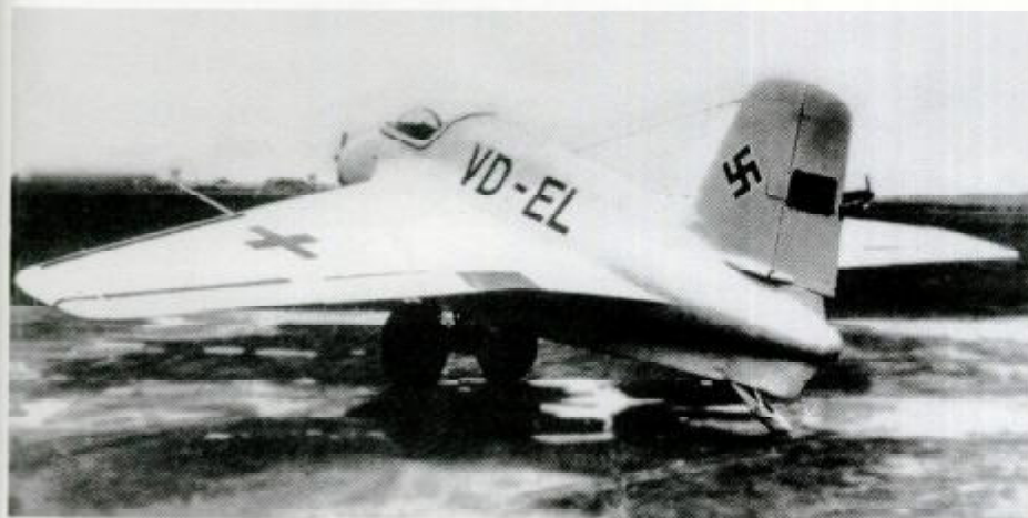
ABOVE: The Me 163 BV2 was the second prototype of the B-series and the first to be fitted with armament and radio equipment. It made its first powered flight on 24 June 1943 piloted by 'Rudi' Opitz.
