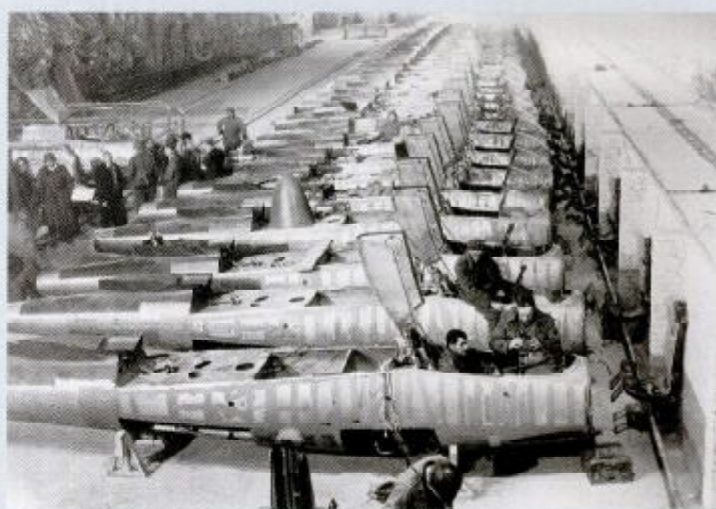
ABOVE: Photographed in April 1945 shortly after its capture by American troops this converted salt mine located at Eger, near Salzburg, was used for He 162 production. At least 40 fuselages can be seen in various stages of completion.
