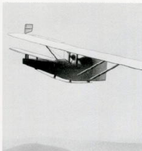
ABOVE: The tail-first Raab-Katzenstein Ente was the first piloted rocket-propelled aircraft to be flown in Germany. After several abortive attempts, the aircraft made its first 60-80 second flight on 11 June 1928 powered by two 20 kg (44 lb) thrust Sander engines. A second flight on that day was abandoned after one of the engines exploded, and set light to the rear fuselage.
