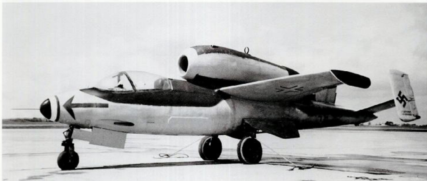
BELOW: The Werknummer (120222) was painted in black on the outside of the vertical tail surfaces of this He 162 A-2 of JG 1. From early 1943, all new Luftwaffe aircraft were allocated six-digit serial numbers.
