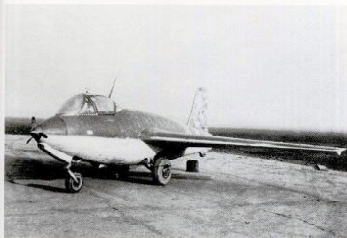
ABOVE: The Ju 248 V1 was completed in January 1945 and test flown as a glider from February. It was an extensively modified version of the Me 163 with a full vision canopy and a fully retractable undercarriage. The prototype failed to fly on the power of its twin combustion chamber rocket engine before the end of the war.
