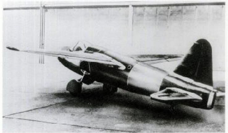
ABOVE: A second prototype of the He 178 was built with an enlarged wing and a fully retractable undercarriage. It was to be powered by the improved HeS 6 engine which was designed to produce 550 kg (1,200 lbs) thrust, but it never flew.
